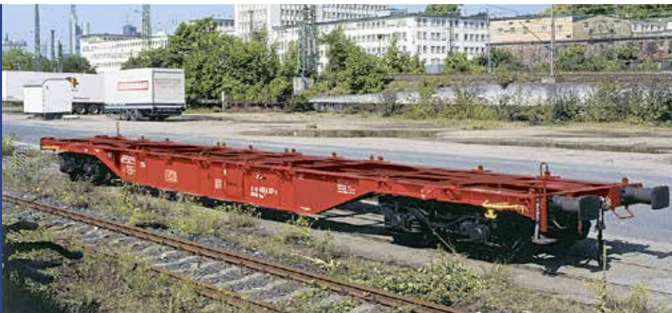
Four-axle flat wagon for large containers and swap bodies Sgns 691
