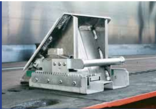
Chocks specially developed by DB prevent paper rolls from moving during transport.
