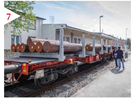
7 — The InnoWagon with steel pallets is the new, weight-optimised, low-noise container wagon from Innofreight.
